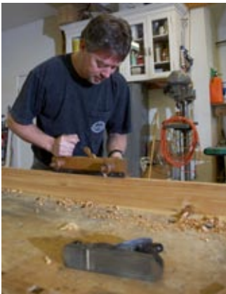
Craftsmen used a historic plow plane to cut grooves for the east wing doors.
