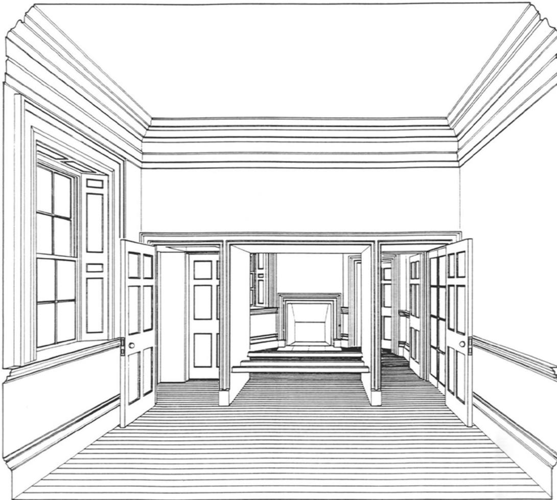
Figure 14. Jefferson proportioned the interior trim and entablatures using proportions from Palladio's Orders with the chair rail as the base. (Mesick Cohen Wilson Baker Architects.)
