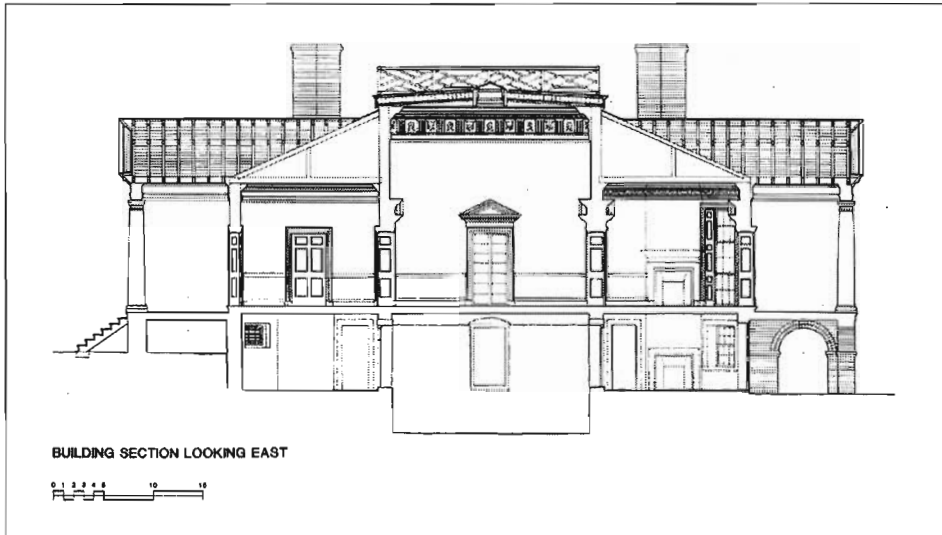
Figure 5. Cross section through Poplar Forest on a north-south axis as seen in this research drawing. Note the higher central dining room with its entablature, skylight and upper Chinese railing; the parlor on the right with its entablature and triple sash windows; and the lower central wine cellar. (Courtesy of Mesick Cohen Waite, Architects)
